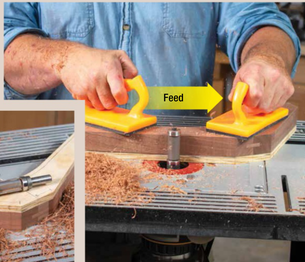
Shape the legs. Fasten the template to the rough-cut leg blank using double-faced tape. Chuck an over-under flush trim bit in your router table and adjust its height so the upper bearing engages the template with the template on top of the workpiece. Start in the center of the curve and feed the piece against the bit's rotation around the end and to the center of the opposite side (left). Then flip the assembly over, adjust the bit height to employ the lower bearing, and trim the other end (right).
