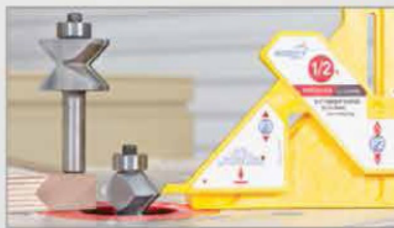
Center router bits and set blade cutting depths.
